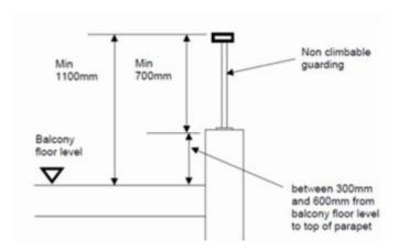
Diagram 2 – Indicates acceptable guarding arrangements where parapet heights are between 300mm and 600mm above balcony floor level. At this height the parapet may be considered as providing an easy step up for a child. Hence a safe non-climbable minimum Barrier height of 700mm needs to be maintained above this level.
