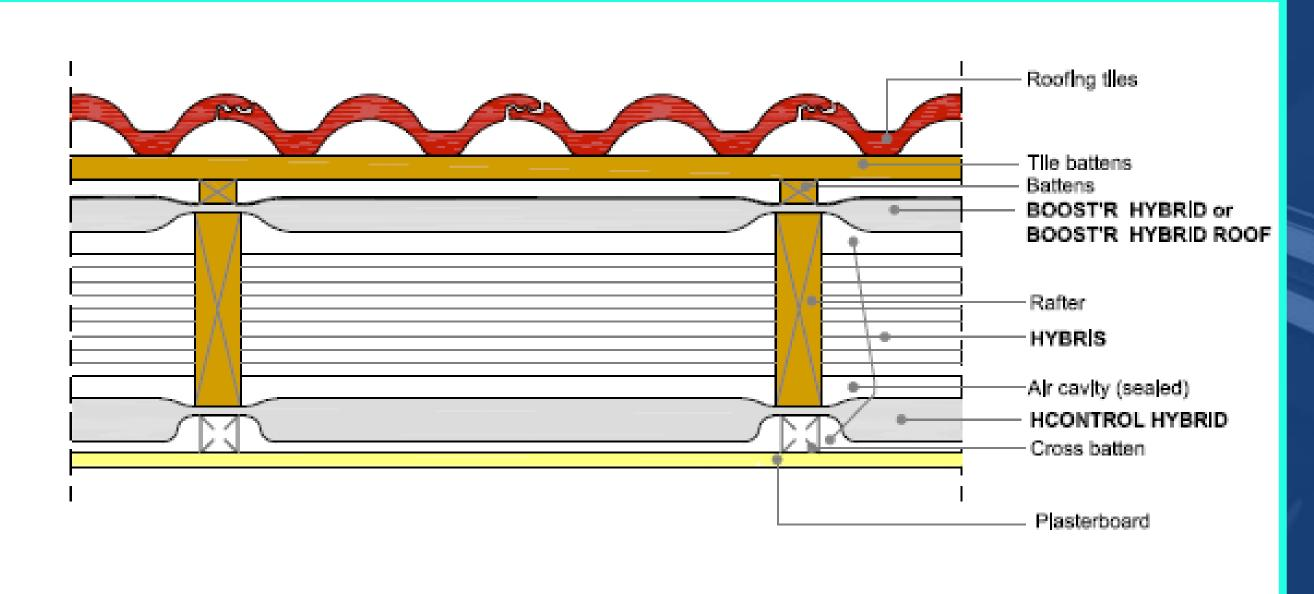
Warm Pitched Roof with BOOST'R HYBRID or BOOST'R HYBRID ROOF HYBRIS Insulation and HCONTROL HYBRID
